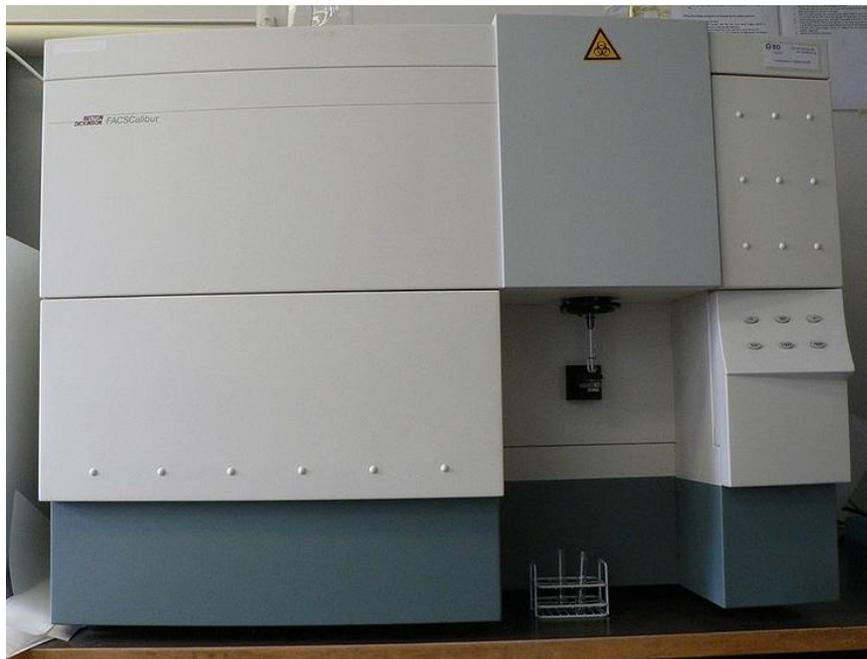
**Figura 4. Citómetro de Flujo** (*Fluorescence activated cell sorter (FACSCalibur)*) (Becton-Dickinson®)
